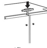
2. Place the provided alignment tool between the doors so that the block sits on top of the doors.
