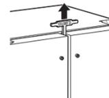
4. Remove the alignment tool. If the gap between doors is uniform, store the tool for future adjustments.
