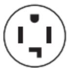
4-wire receptacle (14-30R)
