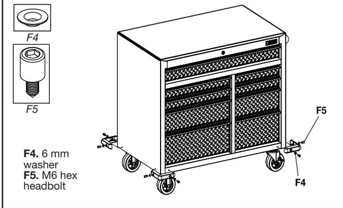
Using 6 mm hex head bolts (F5) (8) and 6 mm washers (F4) (8), fasten a bumper to each corner of the cabinet. Completely tighten all the fasteners.
