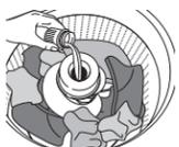
**IMPORTANT:** When using fabric softener, always use the Deep Fill & Rinse to select a setting with '+Extra Rinse' to ensure proper distribution at the correct time in cycle.
