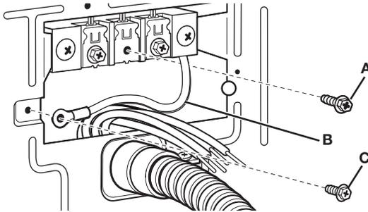
2. Connect neutral ground (B) and place hooked end (hook facing right) of neutral wire (white or center wire) cable under center terminal block screw (B). Squeeze hooked end together. Tighten screw.
