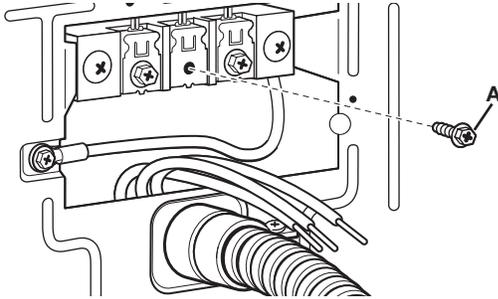
2. Place hooked end (hook facing right) of neutral wire (white or center wire) (D) cable under center terminal block screw (B). Squeeze hooked end together. Tighten screw.
