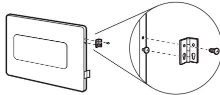
10. Remove the four screws that attach two plugs on the left side. Attach plugs to right side using the same four screws.
