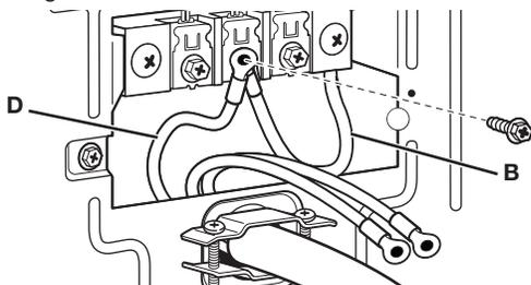
3. Connect remaining wires under outer terminal block. Tighten screws.
