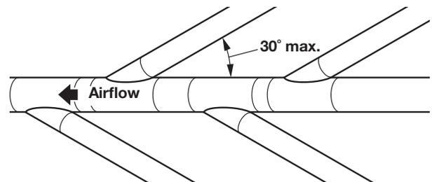
The maximum angle of each vent entering the main vent should be no more than 30°.
