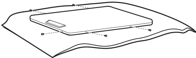
6. Holding door over towel, grasp sides of outer door and gently lift to separate it from inner door. Do not use a putty knife to pry apart. Do not pull on door seal or plastic door catch.
