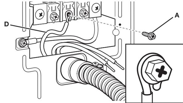
3. Place hooked ends of remaining direct wire cables (hooks facing right). Squeeze hooded ends together and tighten screws. Finally, re-install terminal block cover and tighten hold-down screw. Tighten screws. Go to "Complete Installation" section.
