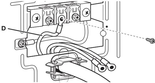
2. Connect remaining wires with outer terminal block screws (F). Tighten screws. Finally, re-install terminal block cover and tighten hold-down screw. Go to "Complete Installation" section.
