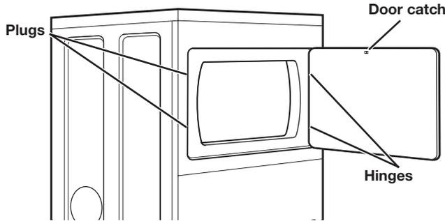
3. Lift door until top screws in cabinet are in large part of hinge slot. Pull forward off screws. Set door (handle side up) on top of towel. Remove top screws from cabinet.
