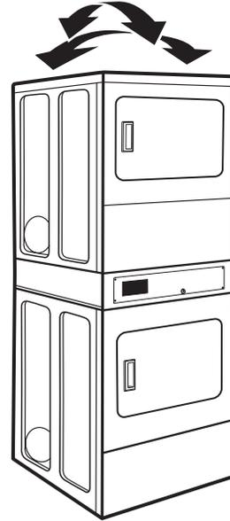
3. If dryer is not level, turn the leveling feet counterclockwise to lower the dryer or clockwise to raise the dryer. Recheck levelness of dryer and that all four feet are firmly in contact with the floor. Repeat as needed.
