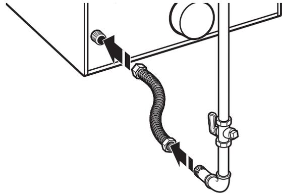
**NOTE:** Do not kink or damage the flexible stainless steel gas line when moving the dryer.
