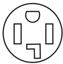
4-wire receptacle (14-30 R)
