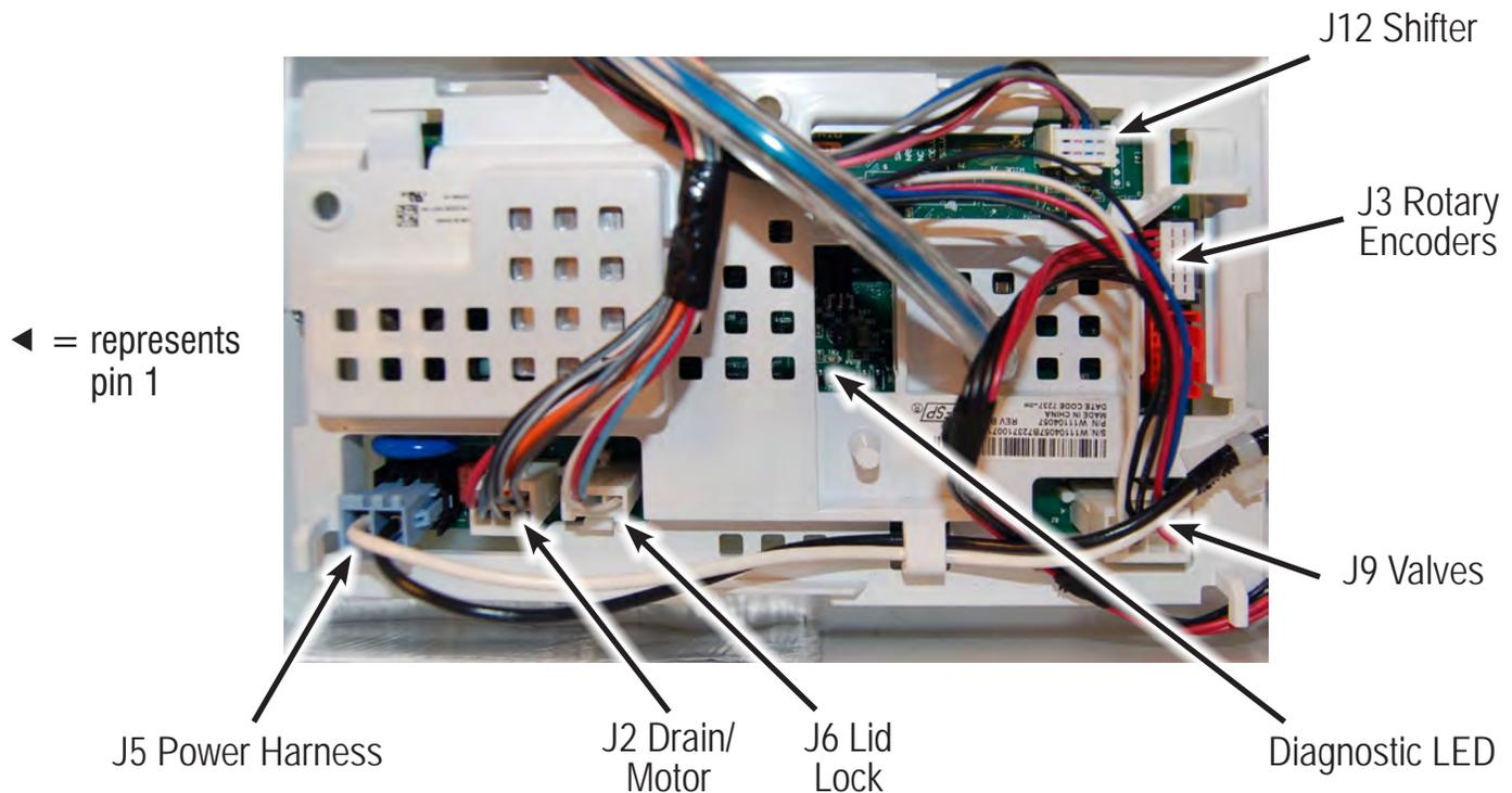
MAIN CONTROL BOARD CONNECTORS AND PINOUTS (FIGURE 2)
