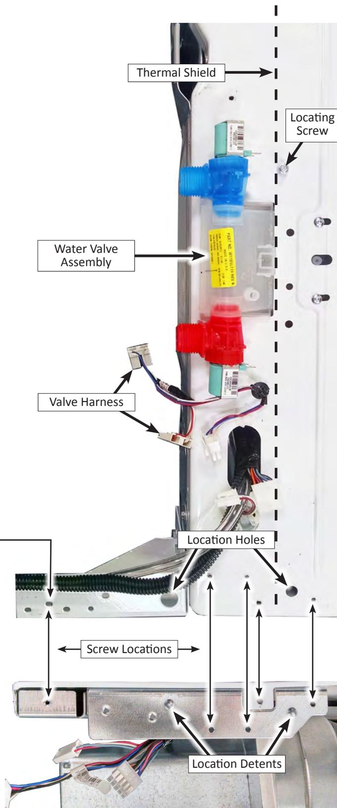
Figure 2 - Dryer Bottom View (one side)
