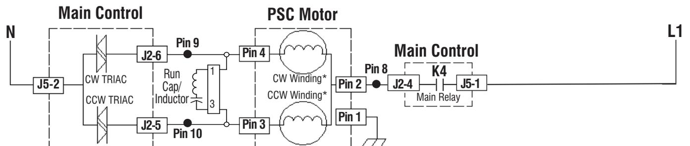
\* 1/3 HP Motor – Each Winding 3.5 to 6 ohms/ \* 1/4 HP Motor – Each Winding 5 to 9.5 ohms
