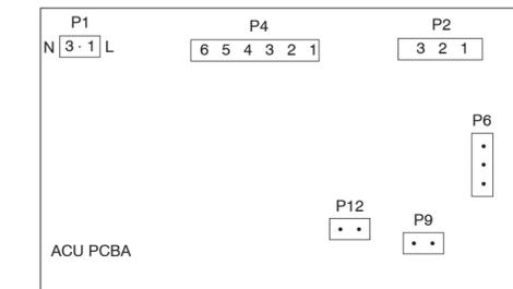
**NOTE:** There are purposely empty terminals between each of the numbered terminals on P1 connectors.
