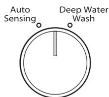
Set the Water Level knob to the Auto Sensing setting and the washer will automatically sense the appropriate water level for the load size and type.
