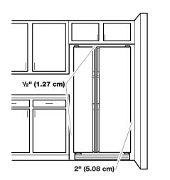
To ensure proper ventilation for your refrigerator, allow for a  $\frac{1}{2}$ " (1.27 cm) space on each side and at the top. Allow for 1" (2.54 cm) of space behind the refrigerator. If your refrigerator has an ice maker, make sure you leave some extra space at the back for the water line connections.
