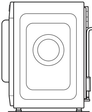
**\*NOTE:** 0"-5" (0 mm-127 mm) spacing is allowed behind dryer, providing drain hose is not kinked or pinched.
