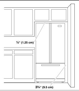
To ensure proper ventilation for your refrigerator, allow for a  $\frac{1}{2}$ " (1.25 cm) space on each side and at the top. Allow for 1" (2.54 cm) of space behind the refrigerator. If your refrigerator has an ice maker, make sure you leave some extra space at the back for the water line connections.
