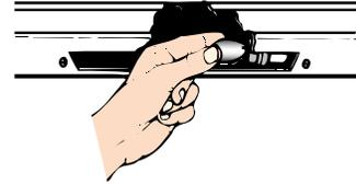
3. Replace bulb with a 40-watt maximum appliance bulb.
