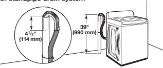
Minimum diameter for a standpipe drain: 2" (51 mm). Minimum carry-away capacity: 17 gal. (64 L) per minute. Top of standpipe must be at least 39" (990 mm) high; install no higher than 96" (2.4 m) from bottom of washer. If you must install higher than 96" (2.4 m), you will need a sump pump system.
