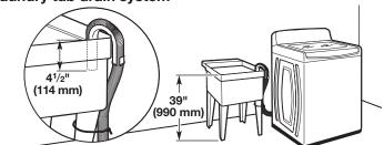
Minimum capacity: 20 gal. (76 L). Top of laundry tub must be at least 39" (990 mm) above floor; install no higher than 96" (2.4 m) from bottom of washer.
