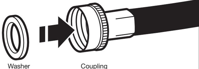
Insert a new flat washer into each end of the inlet hoses (not provided). Firmly seat the washers in the couplings.
