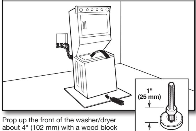
Prop up the front of the washer/dryer about 4" (102 mm) with a wood block or similar object that will support the weight of the washer/dryer. Then screw the locknut onto each foot to within 1" (25 mm) of the foot base.
