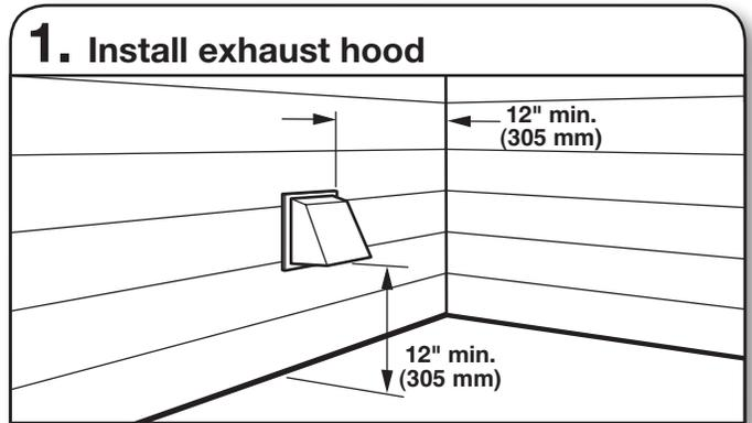
Install exhaust hood and use caulking compound to seal exterior wall opening around exhaust hood.
