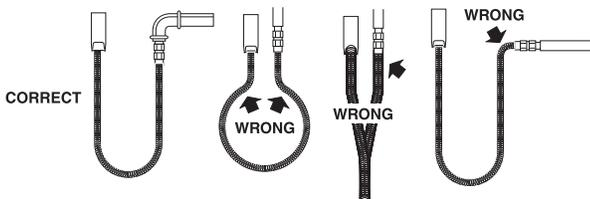
Attach the flexible gas connector to the 1/2" NPT adapter. Do not use pipe-joint compound for this connection.
