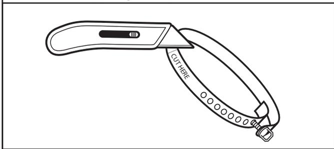
Cut the shipping strap about 16" (406 mm) from the plug end. Look for the words "CUT HERE." Discard end with cotter pins. You will use the remaining piece of shipping strap to secure the drain hose.
