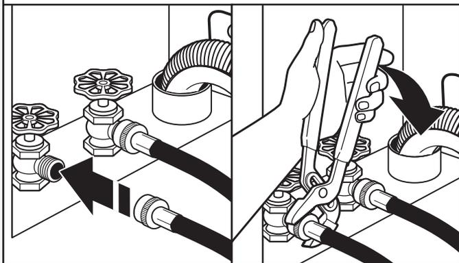
Attach hose to hot water faucet. Screw on coupling by hand until it is seated on washer. Use pliers to tighten couplings an additional two-thirds turn. Repeat this step with second hose for cold water faucet.
