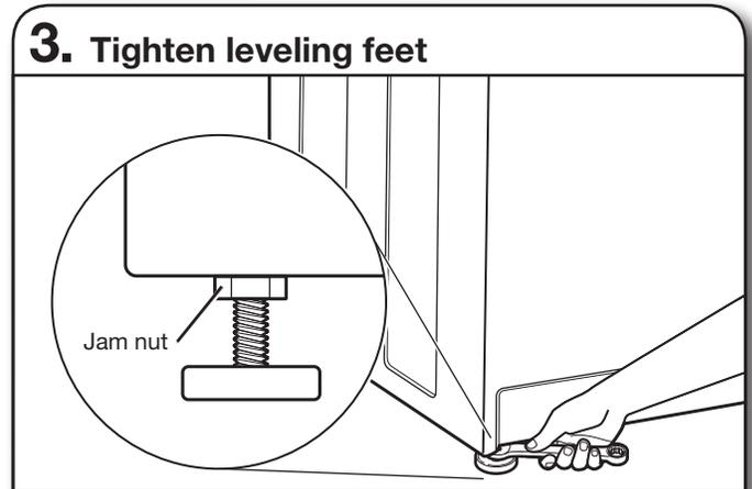
When washer/dryer is level, use a 9/16" or 14 mm open-end or adjustable wrench to turn jam nuts counterclockwise on leveling feet tightly against washer/dryer cabinet.
