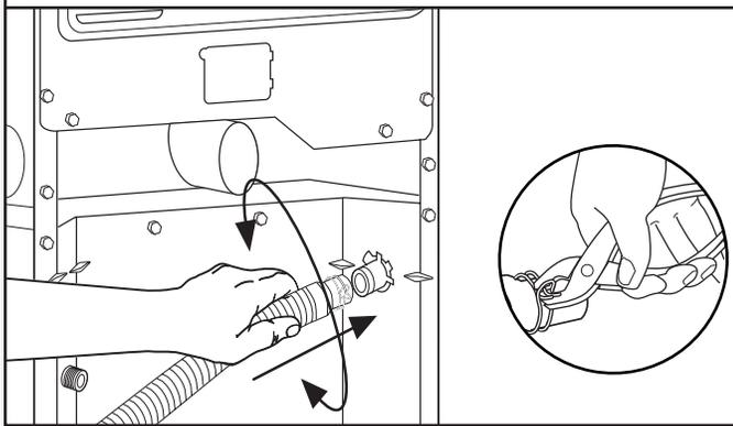
Open clamp. Twist hose back and forth while pushing onto drain connector on the side of the washer/dryer. Continue until hose contacts the ribbed stops on the cabinet. Place clamp over the area marked "CLAMP." Release clamp.
