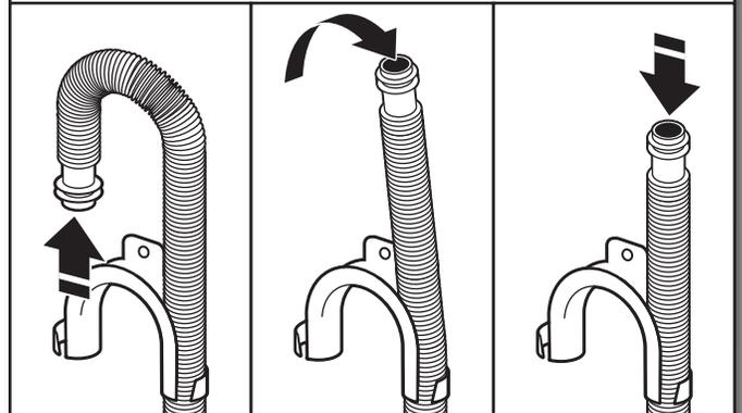
For floor drain installations, you will need to remove the drain hose form from the end of the drain hose. You may need additional parts with separate directions. See "Tools and Parts."
