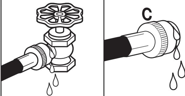
Turn on water faucets to check for leaks. A small amount of water may enter washer. It will drain later.
