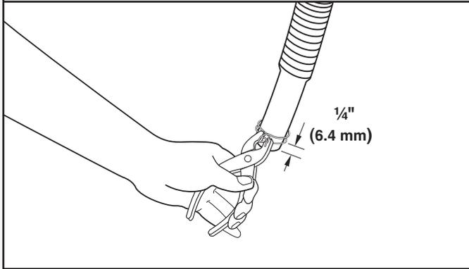
Check the drain hose to see whether it is the proper length. Wet the inside of the straight end of the drain hose with tap water.
