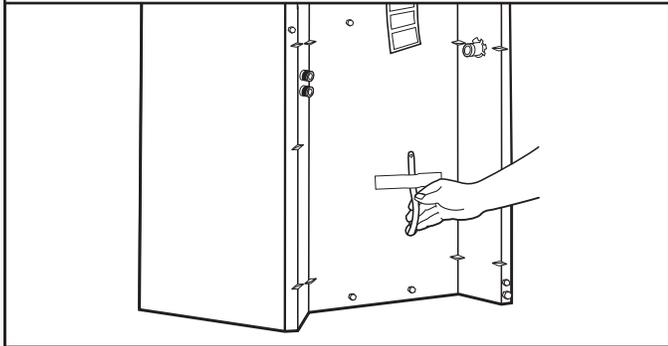
Do not cut yellow strap. Pull yellow strap firmly, until completely removed from washer/dryer. There should be 2 cotter pins on the end of the shipping strap. Remove the hang tag and pin from the vent pipe.
