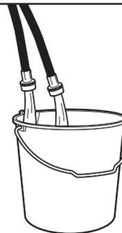
Run water for a few seconds through hoses into a laundry tub, drainpipe, or bucket to prevent clogs. Water should run until clear.
