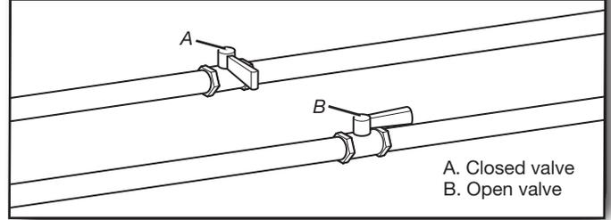
Open shut-off valve in supply line; valve is open when handle is parallel to gas pipe. Then, test all connections by brushing on an approved noncorrosive leak-detection solution. Bubbles will show a leak. Correct any leak found.
