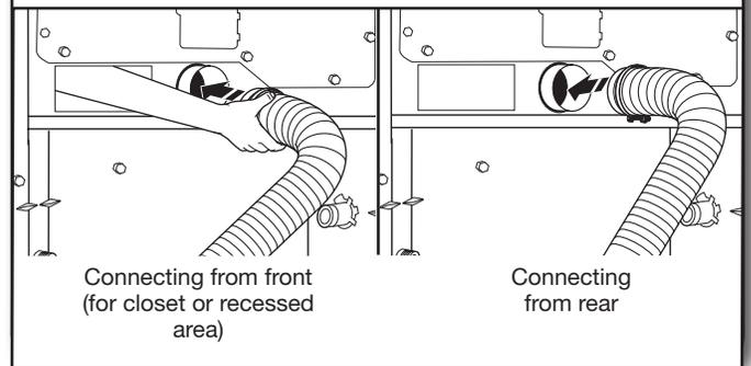
Using a 4" (102 mm) clamp, connect vent to exhaust outlet in dryer. If connecting to existing vent, make sure vent is clean. Dryer vent must fit over dryer exhaust outlet and inside exhaust hood. Check that vent is secured to exhaust hood with a 4" (102 mm) clamp.
