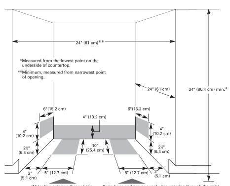
Water line entering through the left side of opening in shaded areas makes connection easier. Minimum ½" (12,7 mm) hole.
