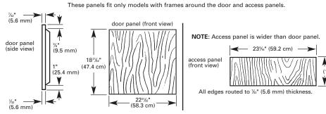
Cut door panel to clear access panel when door is in open position. Custom door panel more than 7/32" (5.6 mm) thick: Rout top and bottom to 7/32" (5.6 mm) thickness.
