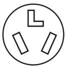
3-wire receptacle (10-30R)
