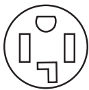
4-wire receptacle (14-30R)
