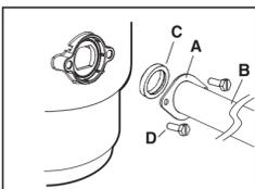
Although the supplied Discharge Tube is preferred, a straight discharge may be used (see Figure 11-2). Slide metal flange (A) over straight discharge tube (B, not supplied), install rubber gasket (C) into discharge outlet, and secure metal flange and straight discharge tube to disposer with two bolts (D).
