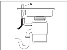
**The disposer installation is now complete.** Run water through disposer and check under sink for leaks. Read **ALL SAFETY INSTRUCTIONS** on next page before operating disposer.
