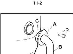
Although the supplied Discharge Tube is preferred, a straight discharge may be used. Slide metal flange over straight discharge tube (not supplied), install rubber gasket onto discharge tube, and secure metal flange and straight discharge tube to disposer with one bolt (reference Figure 11-2).
