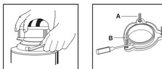
3 DISASSEMBLE NEW DISPOSER MOUNTING ASSEMBLY
