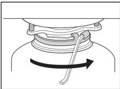
**11 ATTACH DISCHARGE TUBE TO WASTE DRAIN LINE**
