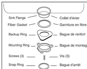
\* Placing a thick, wide rubber band around the sink flange (above the snap ring groove) may help hold parts in place while installing snap ring. (Remember to remove rubber band after snap ring is installed.)
