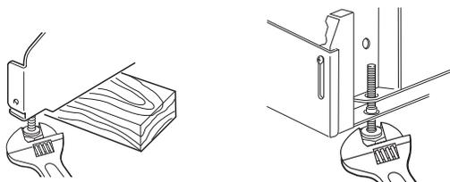
2. Check that leveling legs are firmly against the floor.
