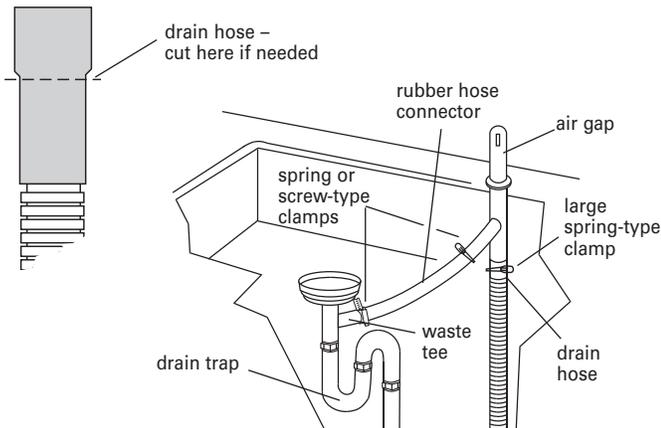
4. Insert drain hose through hole cut in cabinet to the front center of opening where drain connection will be made.
