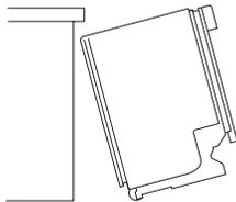
4. If dishwasher has a power supply cord, insert power supply cord into hole cut into cabinet. If using direct wire, check that it is on the right front side of opening.
