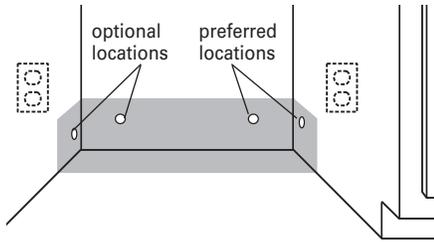
Metal cabinet: Cover hole with grommet (Part No. 302797) included with power supply cord kit.
