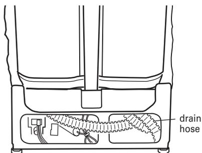
4. The drain hose molded end will fit 5/8" (16mm), 3/4" (19mm) or 1" (25.4mm) diameter connections on the air gap, waste tee or disposer. Cut on the marked line as required for your installation.
