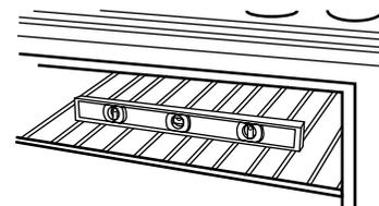
If range is not level, pull range forward until rear leveling leg is removed from the anti-tip bracket.
