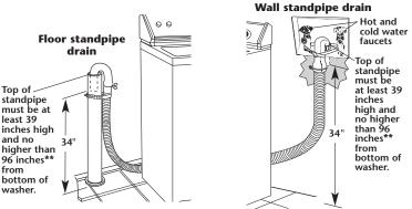
\*\*If the drain height is greater than 96 inches, a sump pump system must be used.
