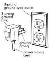
For your personal safety, this washer must be grounded. This washer is equipped with a power supply cord having a 3-prong ground plug.
