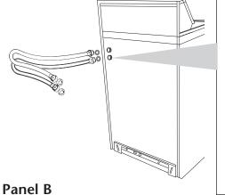
Check inlet hoses periodically. Replace inlet hoses if you find bulges, kinks, cuts, wear or leaking. Replace inlet hoses after five years of use.
