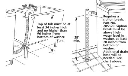
If a longer drain hose is needed, use complete drain hose assembly (56 inches long), Part No. 661575, or drain hose (21 inches long), Part No. 3357090, and Connector Kit, Part No. 285442. These kits are available from your local dealer or an authorized parts distributor.
