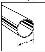
Use 4 inch heavy metal or flexible metal vent. Do not kink or crush flexible metal vent. It must be completely extended to allow adequate exhaust air to flow. Check vent after installation. Refer to your Installation Instructions for proper
