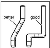
the exhaust vent. Use the fewest number of elbows and turns. Allow room when using elbows or making turns. Bend vent gradually to avoid kinking.
