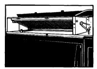
Slide a new charcoal filter into place. The filter should rest at the angle shown.
