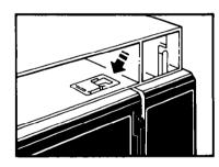
**4.** Remove bulb holder mounting screw.
