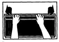
To replace charcoal filter: remove the vent cover mounting screws.
