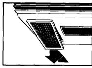
To remove grease filters, slide each filter to the front.
