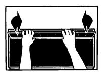
8. Slide the top of the vent cover into place. Push the bottom until it snaps into place. Replace the mounting screws. Turn the power back on at main power supply.
