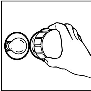
3. Remove the light bulb from its socket.
