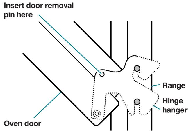
3. Rotate the door toward the range. Lift up the door until it stops. Do not use the door handle to lift the door. Rotate the door toward the floor and pull it toward you.
