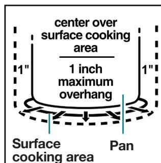
centered correctly, trap heat and can cause damage to the cooktop.
