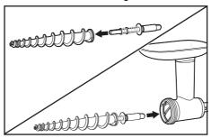
2. Place the Strainer Cone over the Long Grind Screw matching the notch of the Strainer Cone with the tab on the bottom of the Main Housing.
