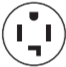
4-wire receptacle (14-30R)
