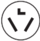
3-wire receptacle (10-30R)
