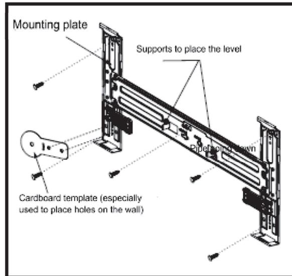
**NOTE:** The shape of the mounting plate may be different from that shown in the illustration, but the installation system is similar.
