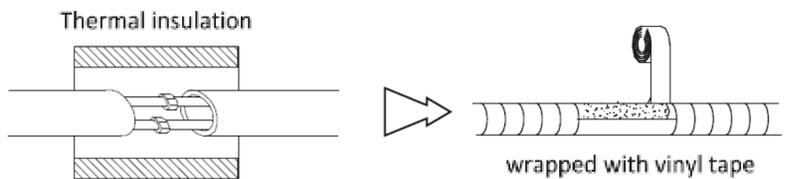
**Thermal insulation on pipes**
