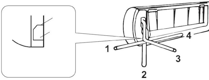
Once the necessary pipe connections have been made, install the drain hose. Then connect the electrical power supply cables. After making the connection, wrap the pipe, cables and drain hose together with thermal insulation material (included in your product).
