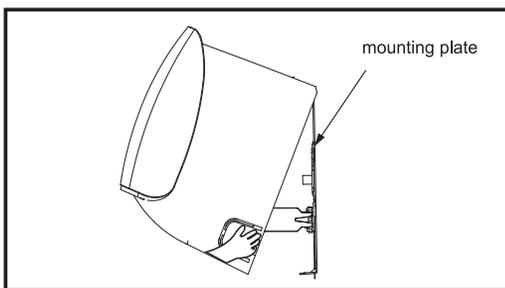
3. Install the indoor unit using the supports
